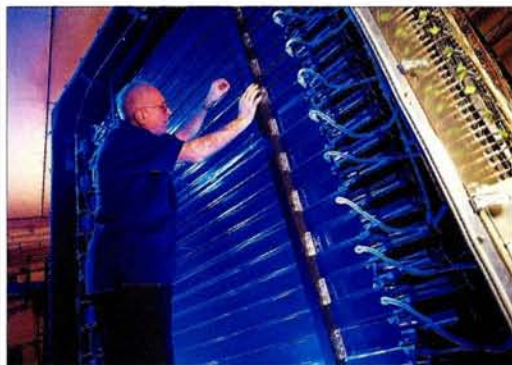
At work on a neutron wall being prepared for use in neutron time-of-flight spectroscopy.
