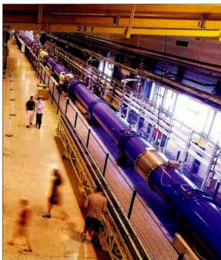
String 2 – a full LHC cell in the regular part of the collider's arc.
